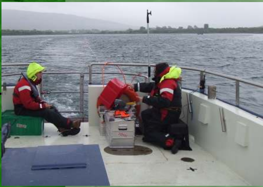
Fig.3: Photo of ERT equipment & cable towed behind boat during Kinvara ERT
